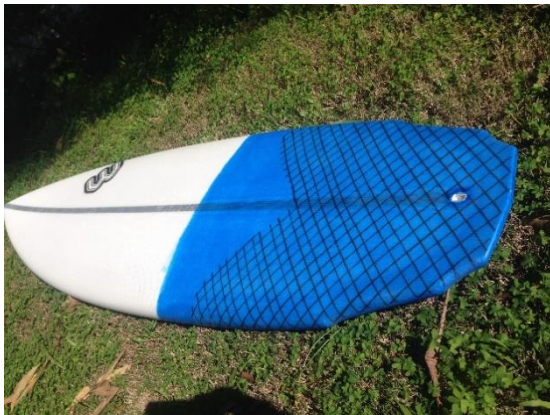
Double flyer, Innegra inlay & quad axial tail patch.
